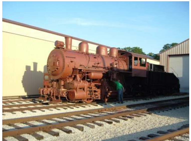
5/27/2010. By the following Thursday, the entire tender has its finish coat of black and the locomotive is in primer.
