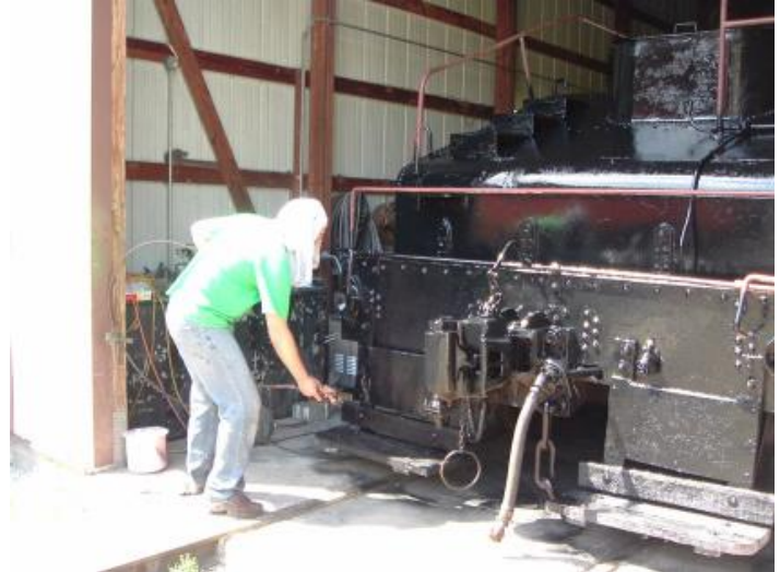
5/23/2010. The next day, the black finish coat is applied to the tender. The coupler has (incorrectly) been painted.
